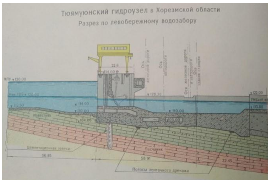
Figure 2-8 A longitudinal profile along the left-bank canal
