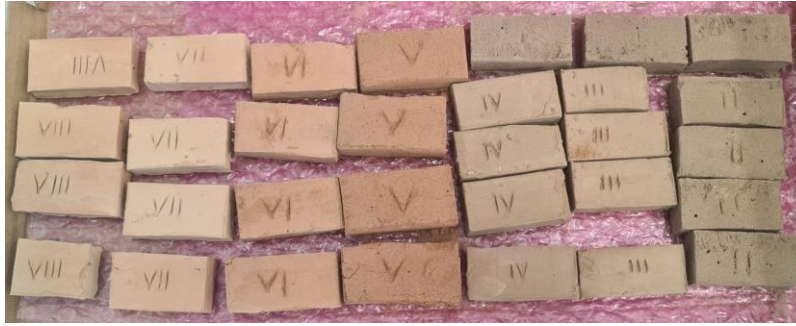
Figure 2-25 The ready sample product (bricks), made using the samples of the Channel reservoir sediment (Central Asian Institute for Ecological Research, 2022)
