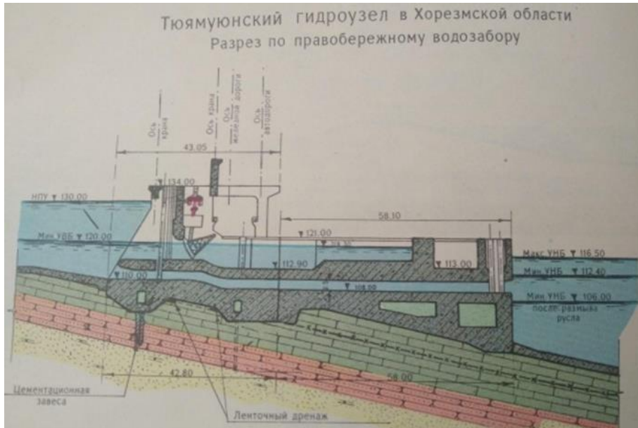
Figure 2-9 A longitudinal profile along the right-bank canal
